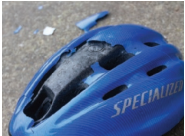
The hard shell of a bike helmet takes some of the force of impact. The dense foam underneath the shell absorbs and distributes kinetic energy, preventing some of it from reaching the rider's skull.
