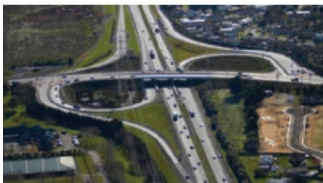
This highway is designed to separate the northbound traffic from the southbound traffic so that head-on collisions won’t occur. Off-ramps are curved, with lower speed limits to prevent accidents. On-ramps are long, to allow for safe acceleration.
