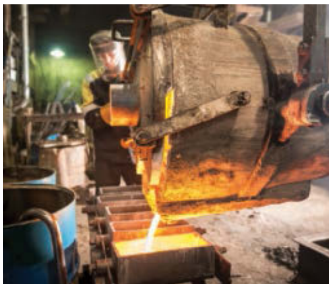
Molten metal is poured into a sand cast. Metal can change state, but no matter is lost or gained in the process.
