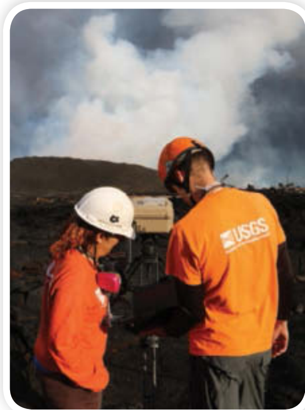
A spectrometer allows geologists to measure the amount of sulfur dioxide in gas plumes released from Kilauea, an active volcano in Hawaii.
