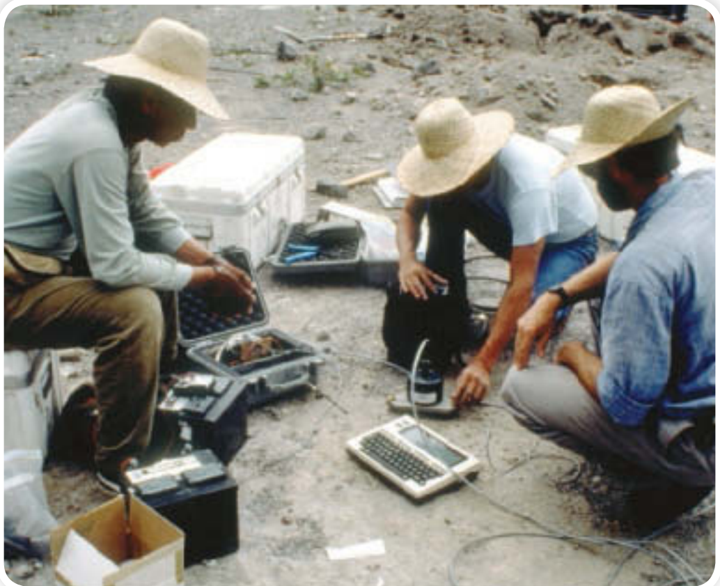
Tiltmeters are devices that scientists use to measure how a volcano moves. This helps them predict when a volcano might erupt.
