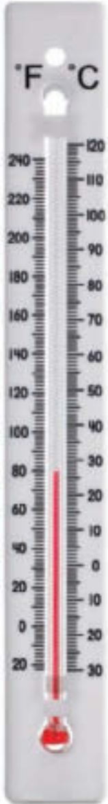
Air temperature is measured with a thermometer.
