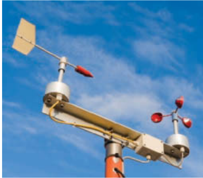
An anemometer, with cups that spin, measures wind speed. A wind vane shows the direction from which the wind is blowing.
