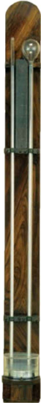
In the earliest barometers, liquid in a tube went up or down with changing air pressure.
